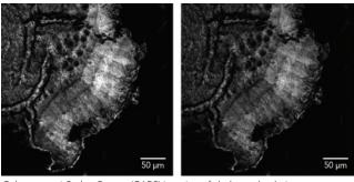
Coherent anti-Stokes Raman (CARS) imaging of cholesteryl palmitate. The image on the left was obtained using Semrock filter FF01-625/90. The image on the right was obtained using a fluorescence bandpass filter having a center wavelength of 650 nm and extended blocking. An analysis of the images revealed that the FF01-625/90 filter provided greater than 2.6 times CARS signal. Images courtesy of Prof. Eric Potma (UC Irvine).
