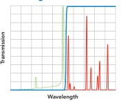
Laser-blocking steep edge filter for superior Stokes measurements.
