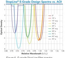
Figure 4: E-grade StopLine filter spectra.
