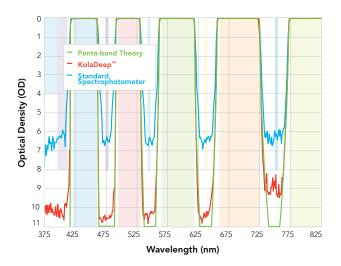
The graph below shows spectral performance for a custom hexa-notch filter designed to ensure precise blocking of six laser lines. This customer required assurance that each laser line is repeatably blocked at a specific level. The spectra measured with our KolaDeep SMS show precise matches to the specifications, even in the UV region. The measured blocking (red) matches theory (green).
