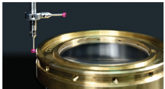
Unequaled repeatability and scalability result from integrated metrology in the ATS 200 alignment turning machine (photo courtesy of TRIOPTICS GmbH)
